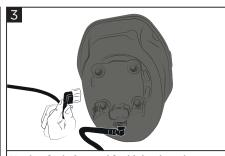
Unplug fuel pipe and fuel injection plug. Then drain the fuel tank.
