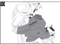
Install the fuel tank (A) by reconnecting fuel pipe and fuel injection plug. Then tighten using washer (B) and screw (H) and hook with the rubber band (S), paying attention to hook it first on the tank's bracket and then on the bike's frame.
