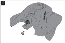
Insert grommet (D) ad bushing (C) in the
