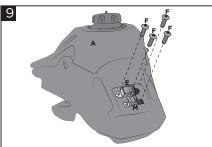
Mount the brackets (E) and (M) through screws (F).
