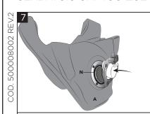
Insert the O-ring (N) in its seat on the Acerbis fuel tank (A).
