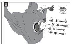
Mount the bracket (T) and tighten using the bushings (R), the original washers (Q) and the provided screws (G).
