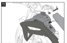
Reassemble the radiator shrouds using washer (I) and screw (L). Then remount the saddle.
